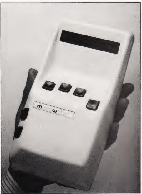
The Microwriter is a handheld word processor with only five keys. Now it can speed up text entry on the BBC.
